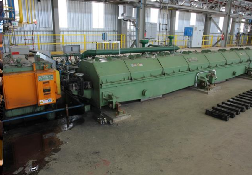
HYQST Traversing Water Box Arrangement
