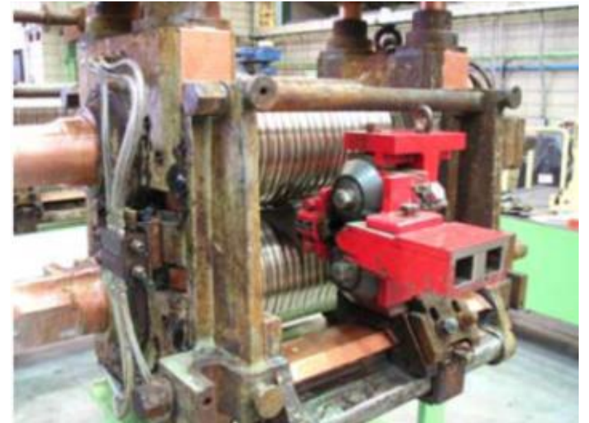
Typical Slitting Guide Arrangement
